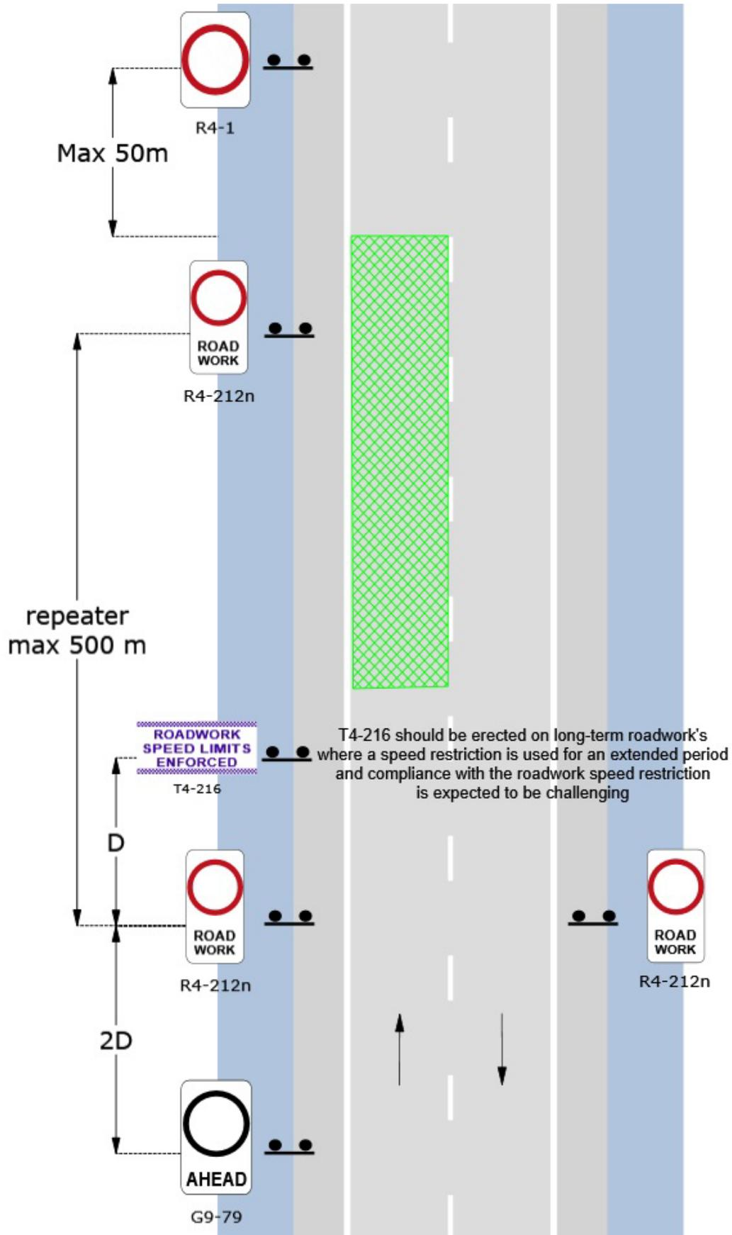
D.4.10 Static: Use of temporary portable rumble strips (shuttle flow)
