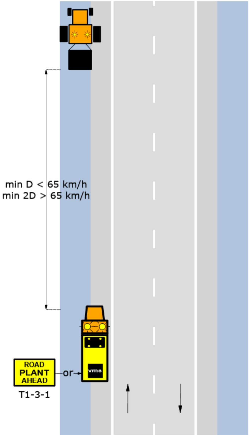
D.4.16 Dynamic: Continuous work, grading - 2 lane / 2 way (formerly TCP 105)
