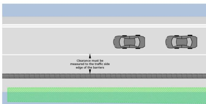
Figure 6-2. Clearance measurement from delineating device (barrier)
