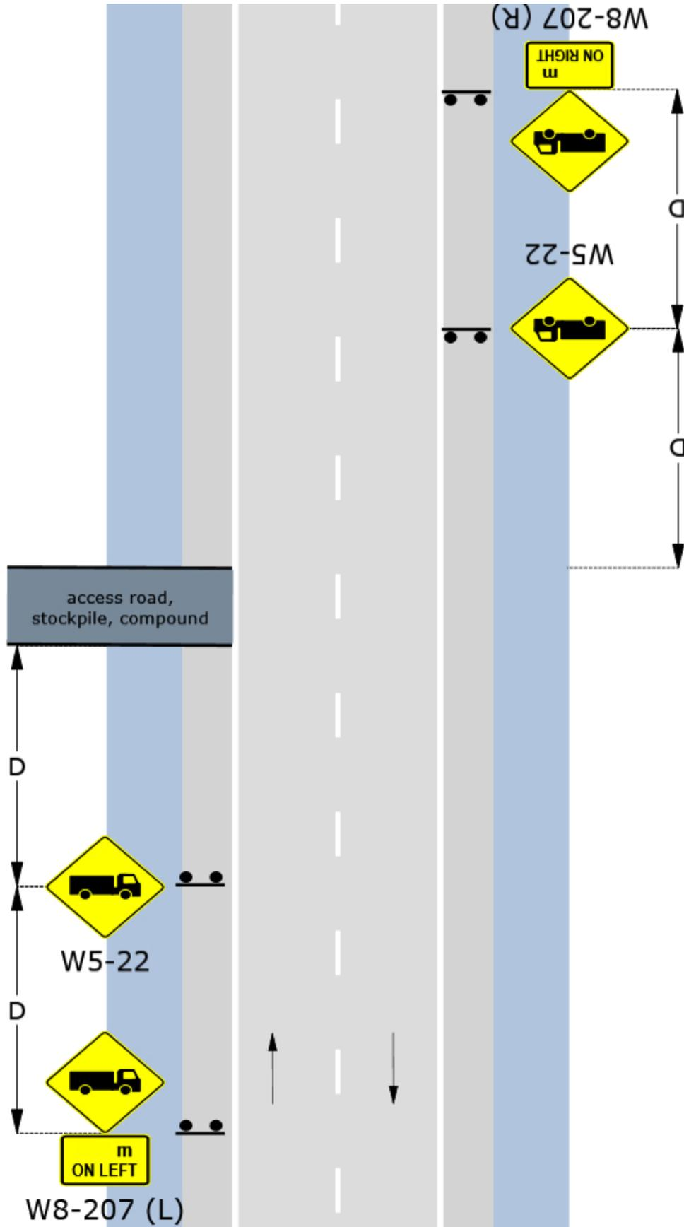
D.4.8 Static: Bitumen sealing - 2 lane / 2 way (formerly TCP 95)
