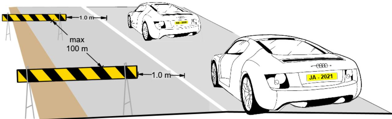
Figure 6-31. Typical example of a barrier board
