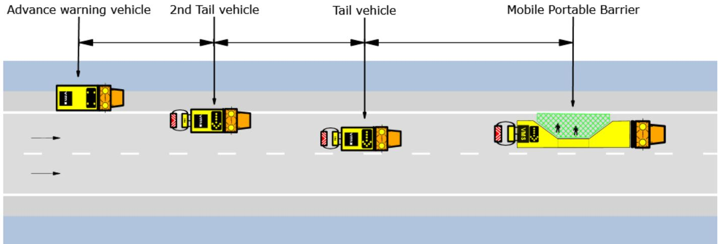
Figure 6-30. Example of a mobile safety barrier
