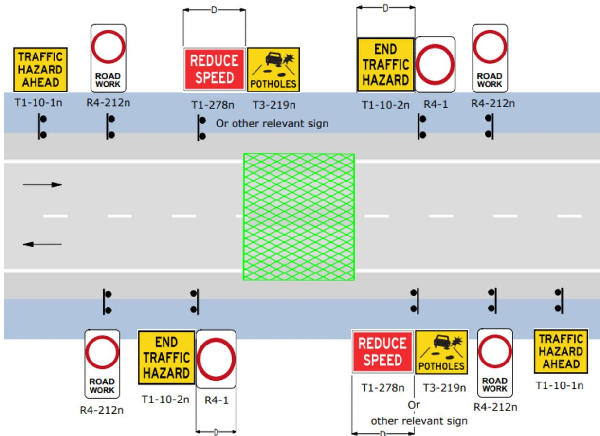
Figure 7–15a Example layout – sign posting a traffic hazard
