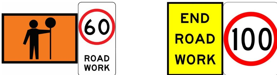
Figure 6-6. Side-by-side dual sign arrangements
