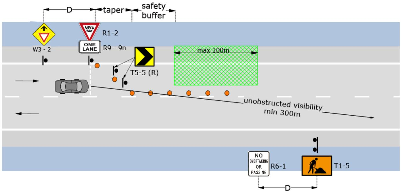
Figure 7-11. Example layout – single lane operation
