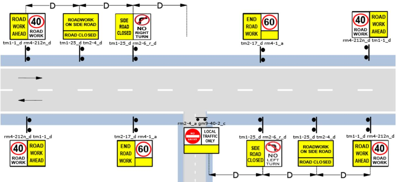
Figure 6-9. Typical MMS layout – side road closed
