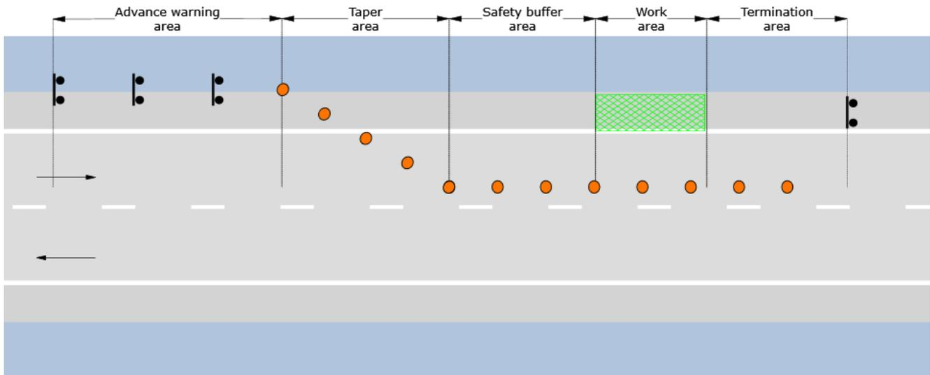
Figure 7-3. Components of a work site
