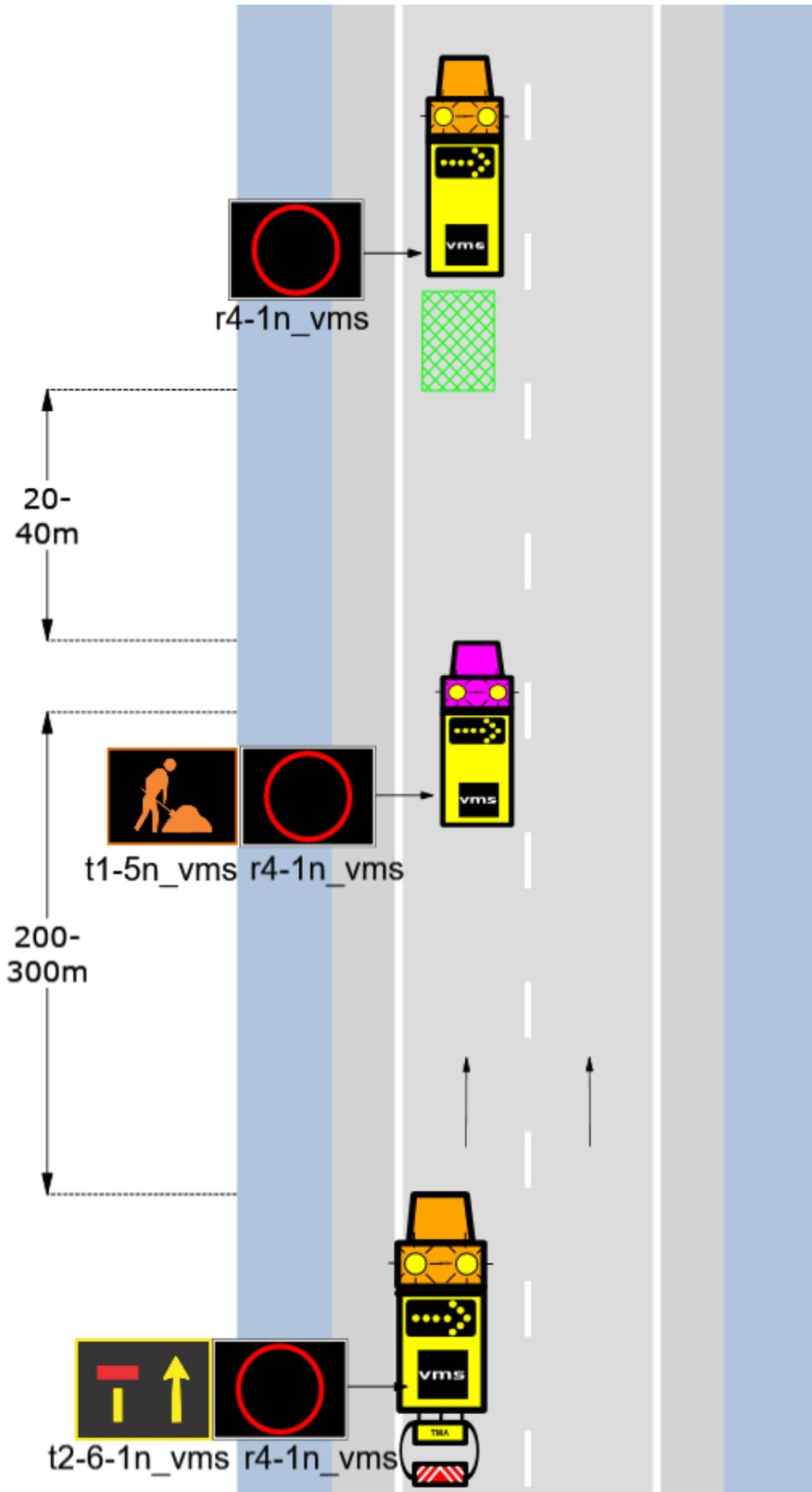
D.4.14 Dynamic: Continuous work in traffic - 3 lane / 2 way work (formerly TCP 70)
