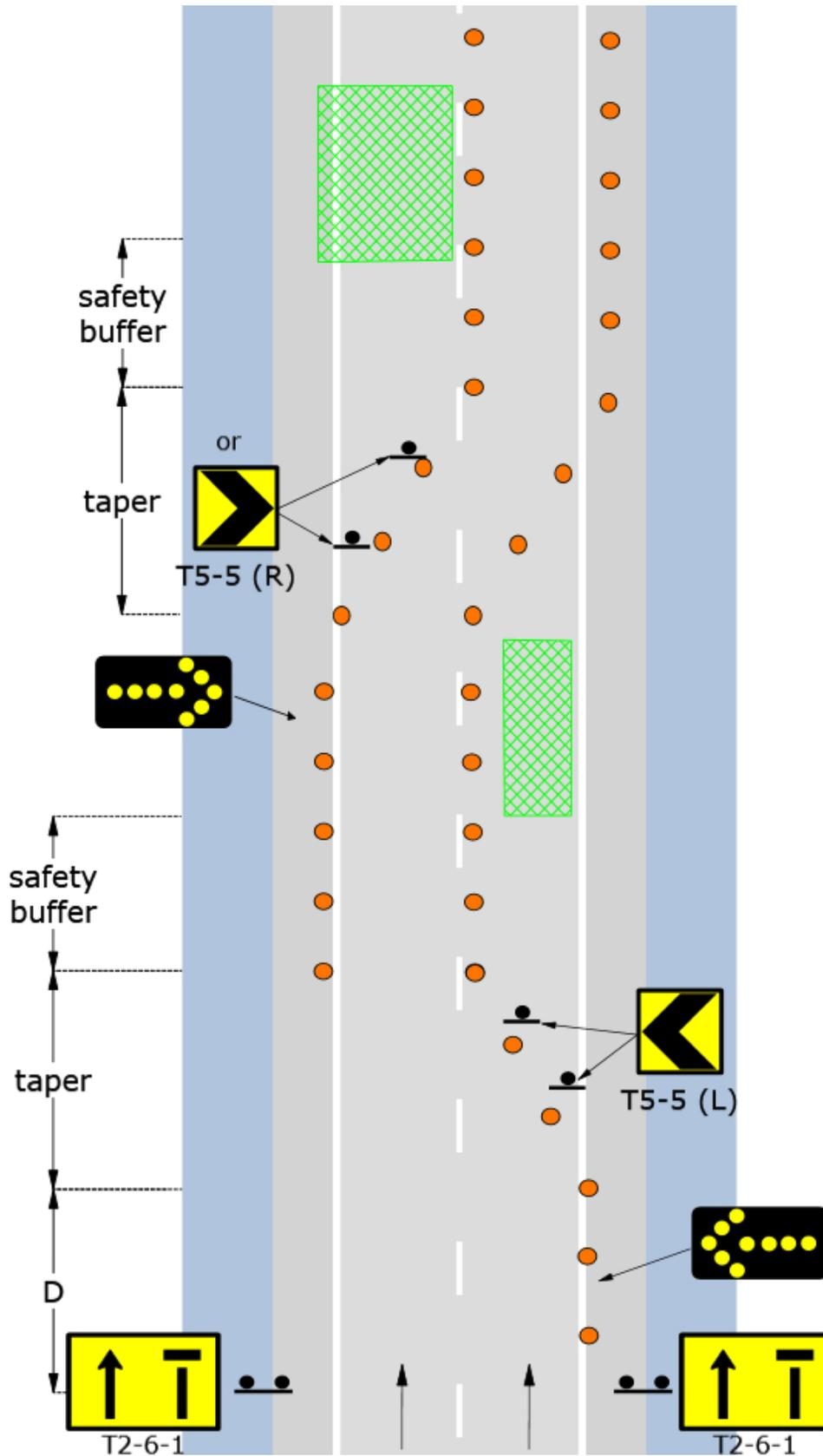
**D.4.2 Static: Lane closure with double chicane – 2 lane/divided (formerly TCP 102) – left to right merge**
