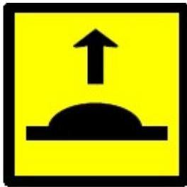
Figure B-12. T5-210 Speed hump ahead sign
