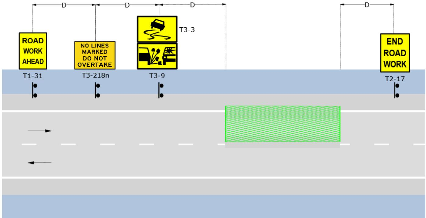
Figure 7-14. Example layout – bituminous works
