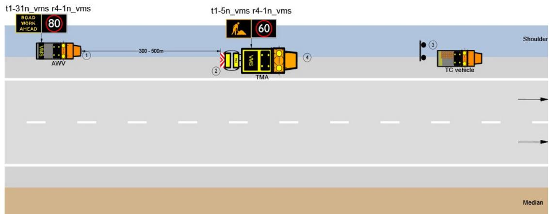
**Figure 6–11 Removal stage 3: Advance warning area**
