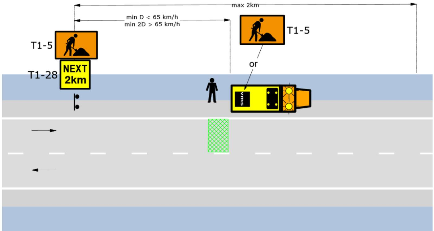
Figure 7-17. Example layout – frequently changing work
