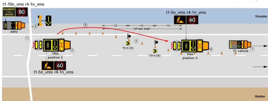
**Figure 6–7 Installation Stage 3: Taper and lane closure**
