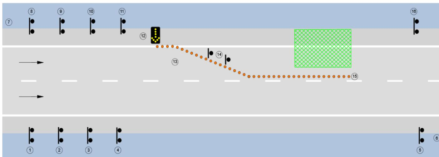
Figure 6-4. Example sign installation sequence for a multi-lane road
