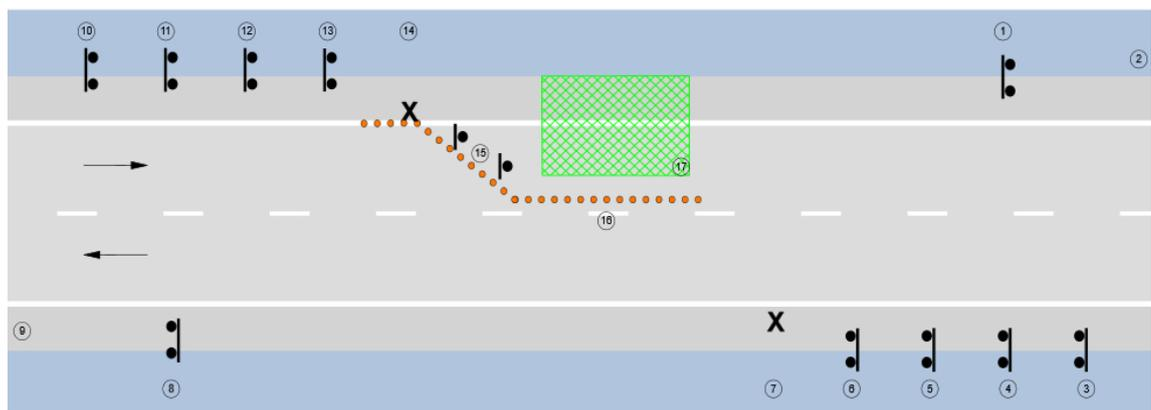
Figure 6-3 Example sign installation sequence for a two-lane, two-way road
