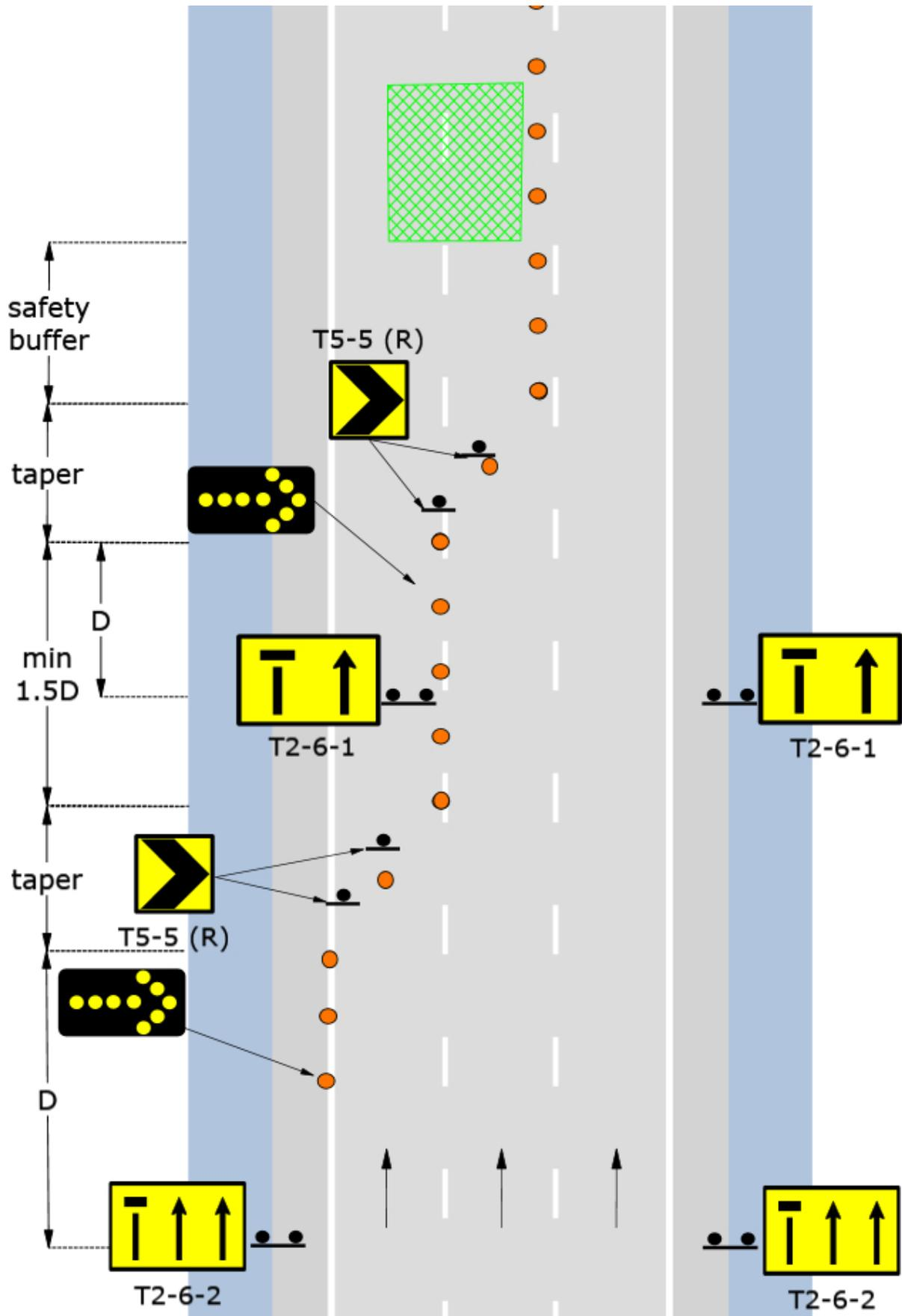
D.4.4 Static: Dual lane closure for work in fast lane - 3 lane / 2 way (formerly TCP 90)
