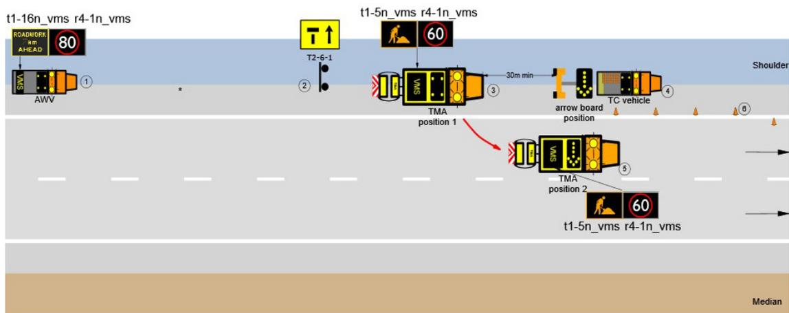
**Figure 6–6 – Installation Stage 2: Arrow board and pre-taper**
