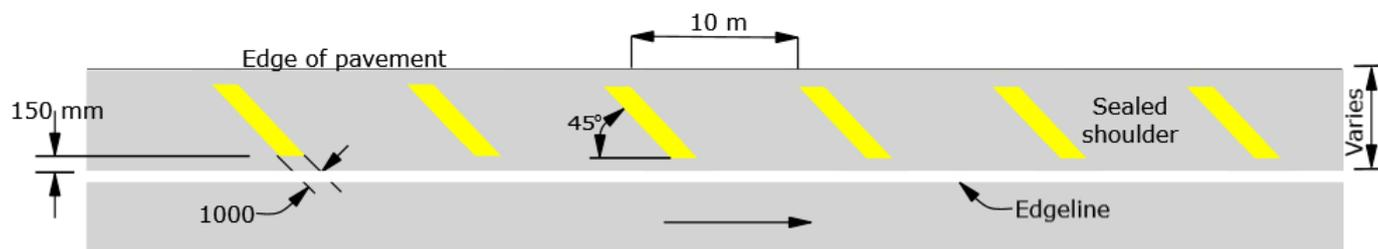
Figure 5-2. Required yellow linemarking and diagonal marking dimensions, spacing and angles
