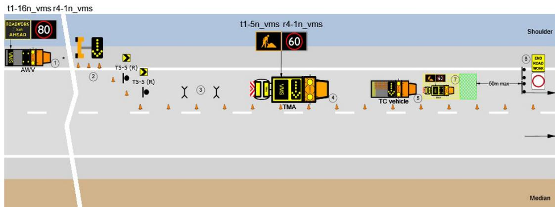
**Figure 6-8 Installation Stage 4: Lane closure and end roadworks**
