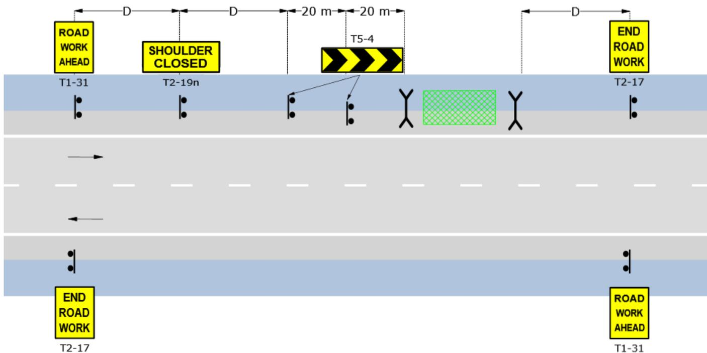
Figure 7-10. Example layout – shoulder closure
