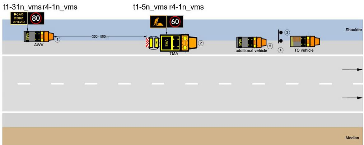
**Figure 6–5 – Installation Stage 1: Advance warning area**
