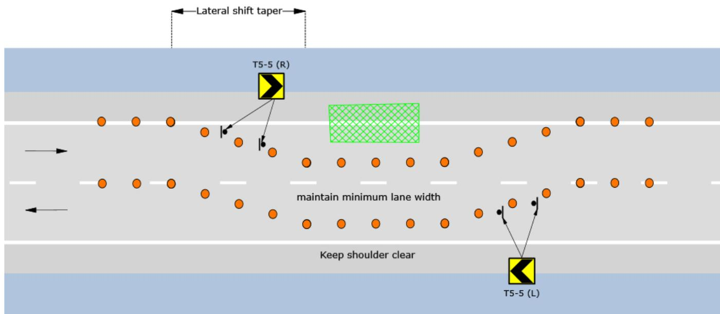
Figure 7-9. Example layout – static: lane closure, two-lane, two-way (formerly TCP 41)
