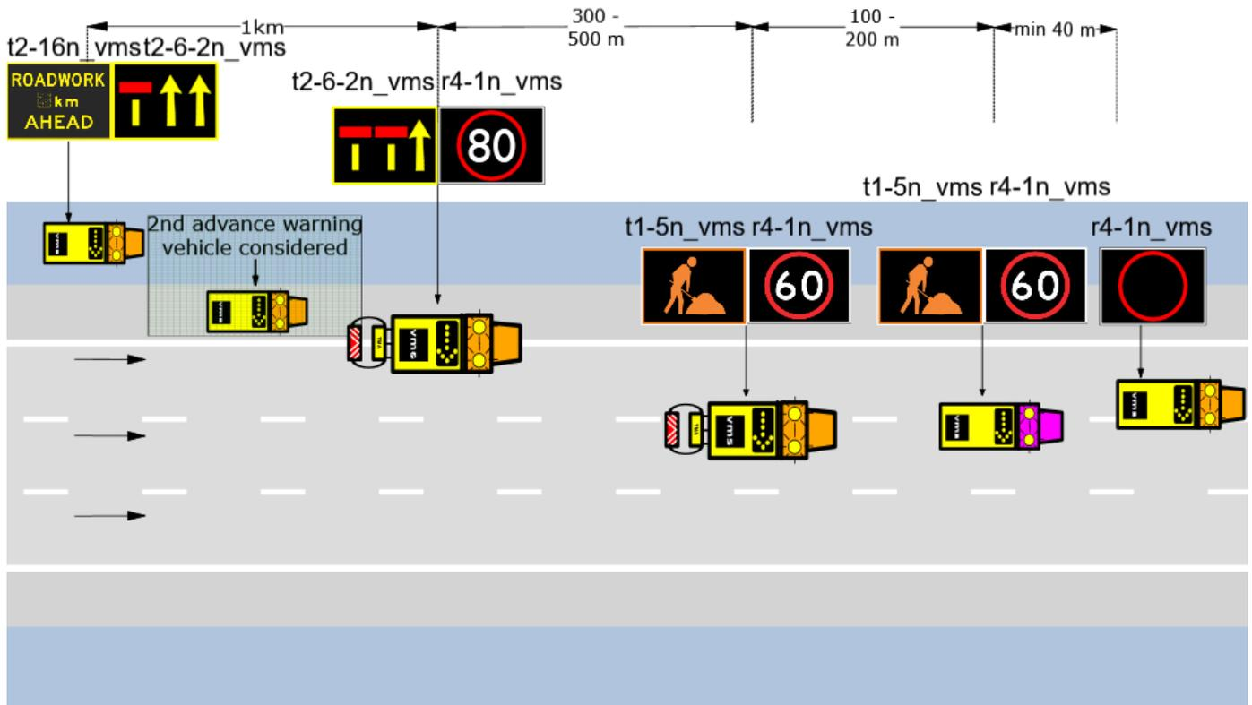
Figure 7-19. Example layout – continuous work
