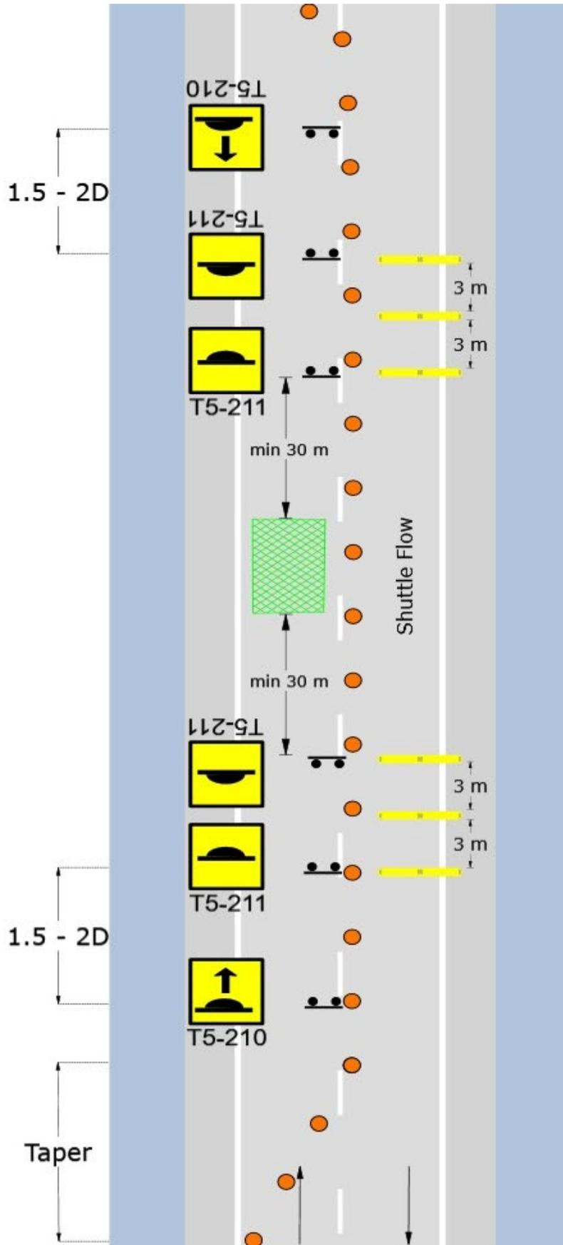
D.4.11 Static: Use of temporary portable rumble strips (merge lane closure)
