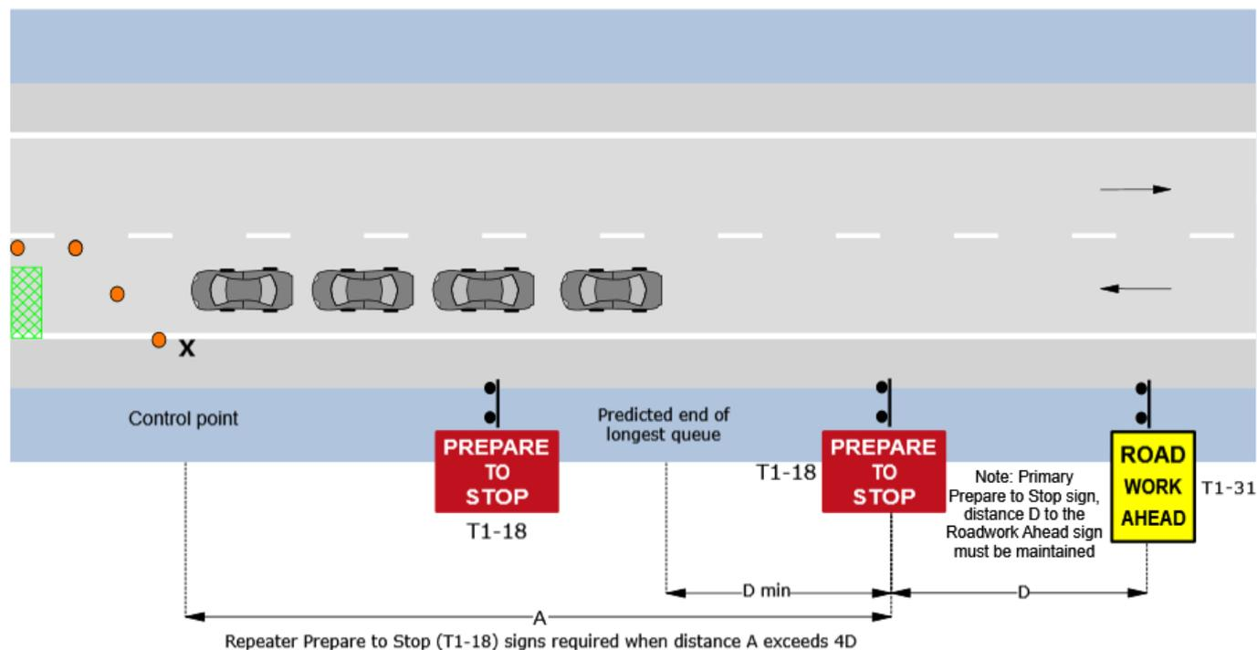
Figure 4-4. Avoiding end-of-queue collisions example
