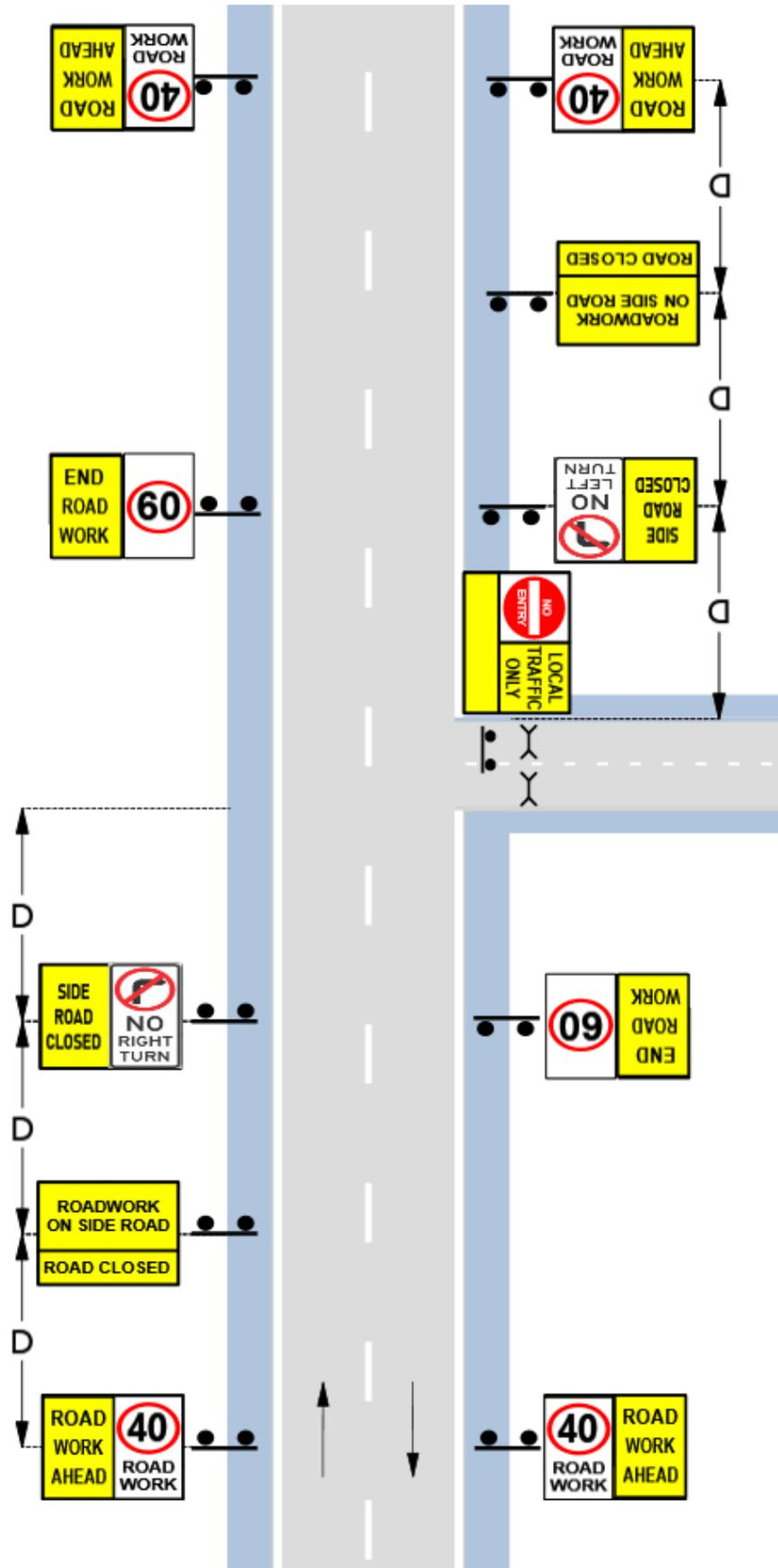
D.4.7 Static: Access to depot, stockpile, quarry, gravel pit etc. all roads (formerly TCP 195)
