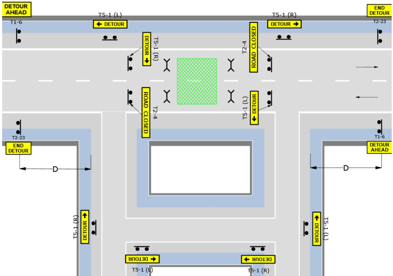
Figure 7-7. Example layout – detour
