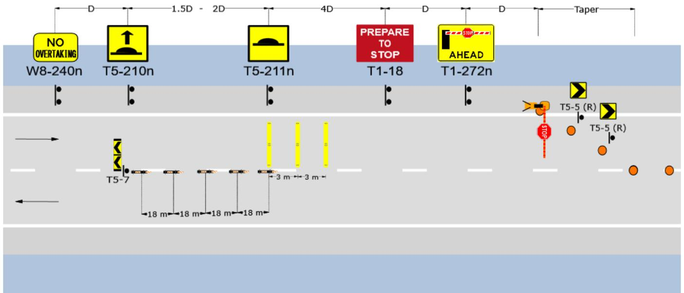
Figure 6-38. TPRS layout – boom barrier
