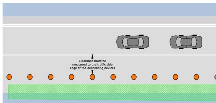
Figure 6-1. Clearance measurement from delineating device (cones)
