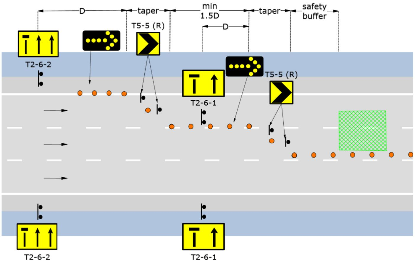
Figure 7-12. Example layout – static: lane closure, 3 lane
