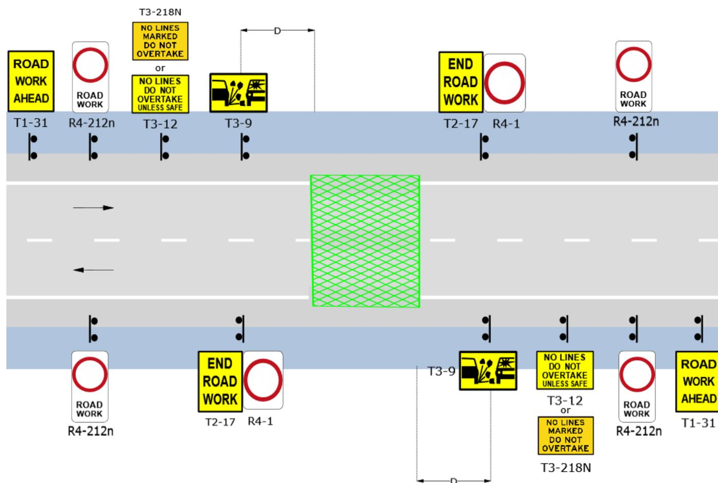
Figure 7-15. Example layout – aftercare
