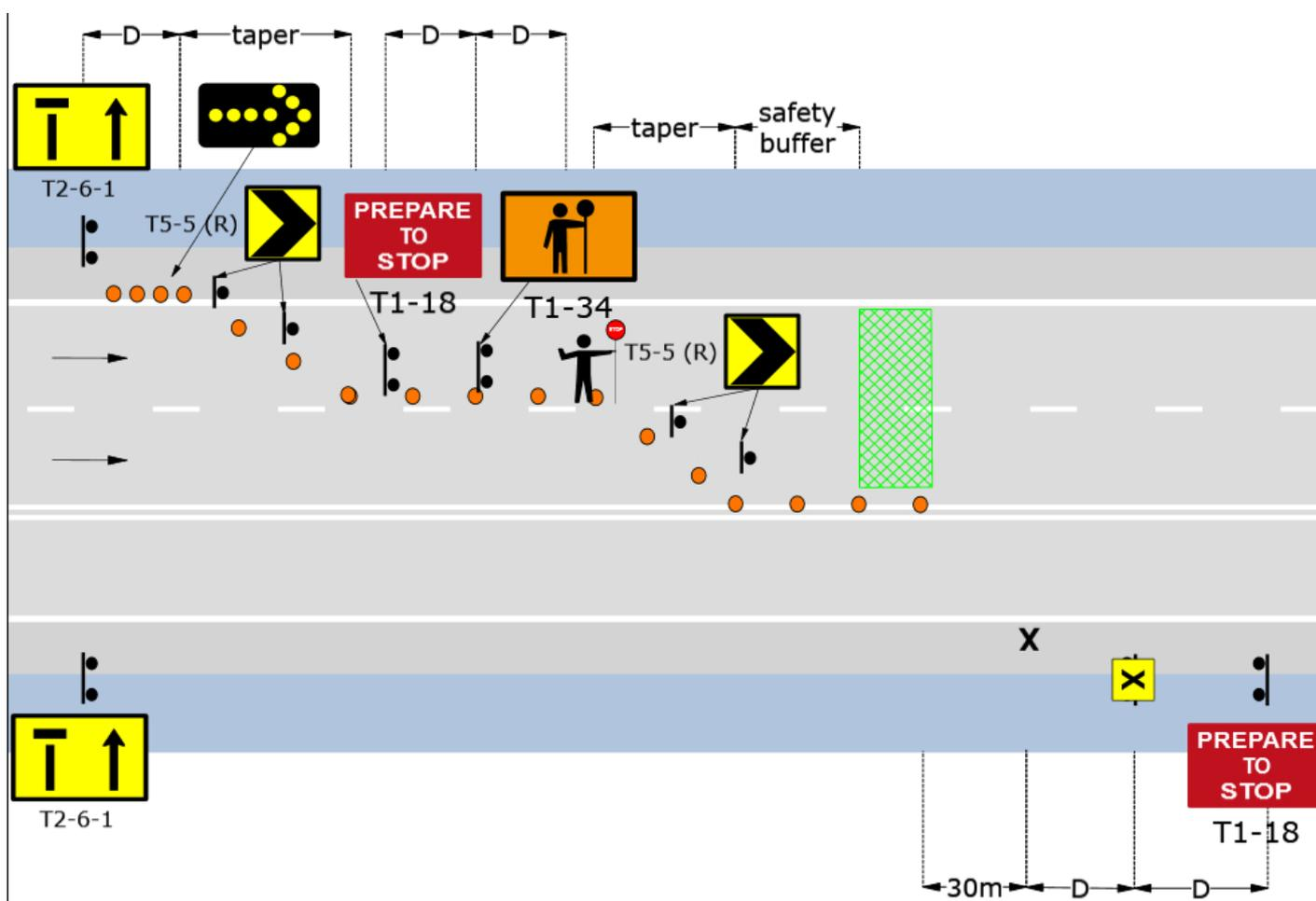
Figure 5-4. Manual traffic controller for multi-lane carriageway
