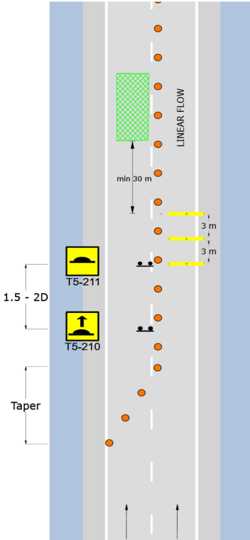
**D.4.12 Dynamic: Continuous work - use of truck -mounted attenuator**
