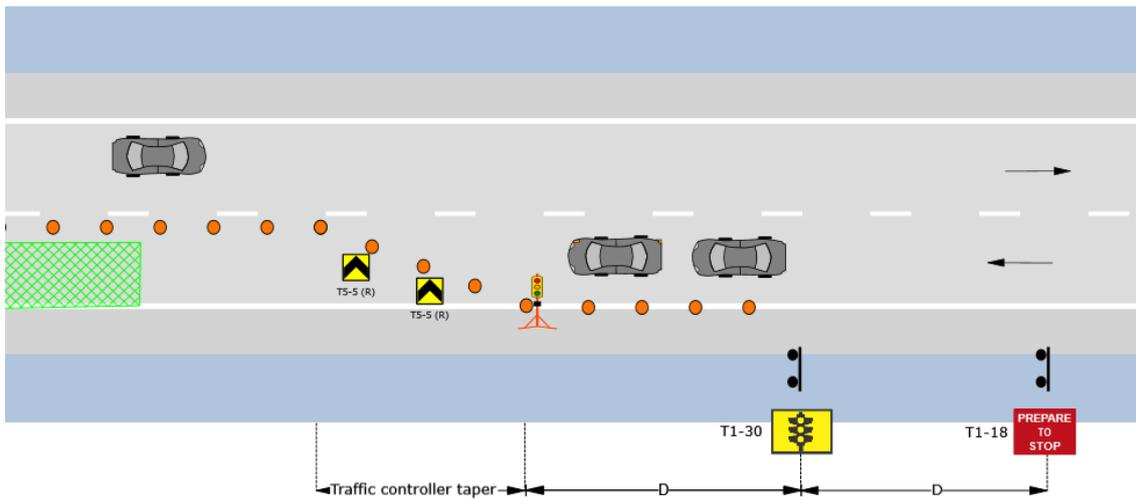
Figure 7-4. Traffic control taper with Type 1 PTS
